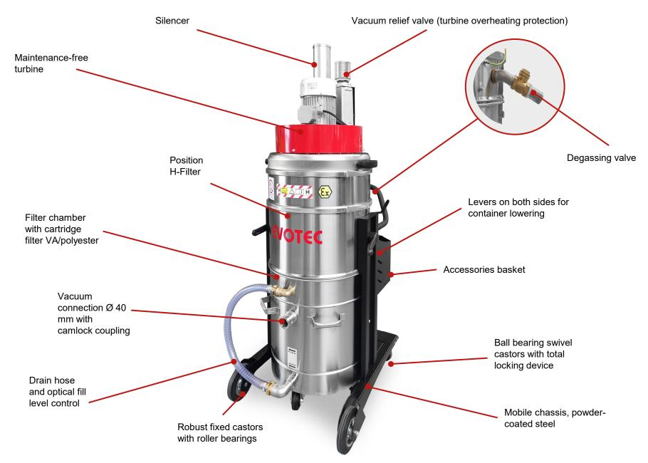
Powerful industrial vacuum cleaner with liquid bath separator integrated in the dirt container for the extraction of explosive, deposited metal dusts such as aluminium, copper, titanium.
